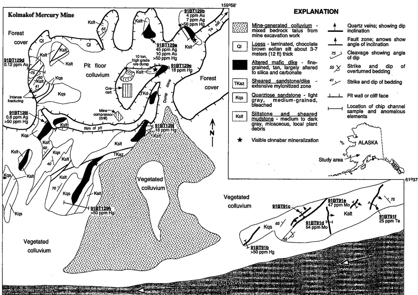
FIG. 17. Geologic sketch of the Kolmakof mercury mine, Sleetmute C-8 quadrangle, illustrating precious metal-bearing mineral zones in a Kuskokwim mercury lode. Data from this study. Sketch by T.K. Bundtzen and G.M. Laird, June 22, 1991.
